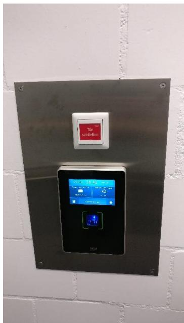
Activate the goods lock with an authorization on the fingerprint terminal. Open the door fully until it holds by itself.
